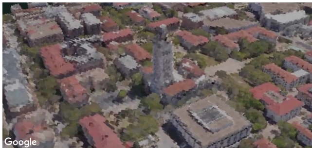
Figure 4. UT Austin Tower voxelized at low resolution. Lowering voxel resolution represents the same structure with less data.
